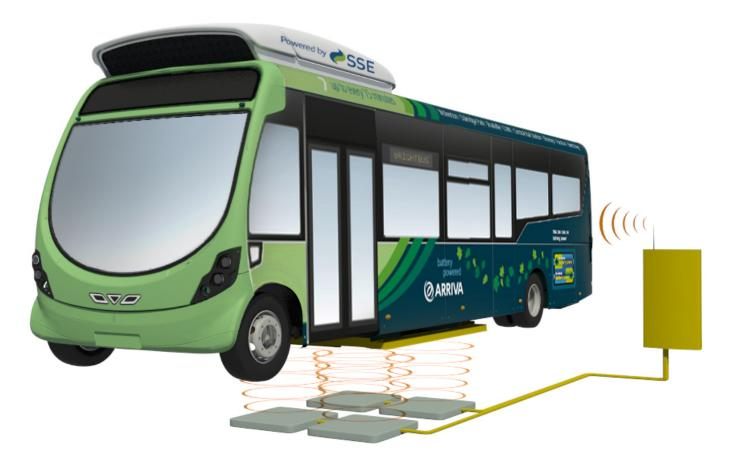
IPT-Tech (Conductix-Wampfler) 4x30kW = 120kW 20kHz, liquid cooled
